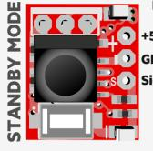
+5V At open mode, Microstart waits for pushing remote's GND (-) (release) unlock button. At that state both leds turn off. When you push the release button of remote, signal output Signal of remote will stay on OV when you push the start button signal go from OV to 5V (Logic 1) and it will stay at that situation. And blue led lights. When you push the stop button, signal output will go from 5V to 0V (Logic 0) and red led will light.
