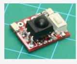
Easy to use start module for mini sumo robots, sumo robots. You can use any three buttons of Sony remote with Microstart. (Release, Start, Stop) For signal output, you need to save remote signals to module first.
